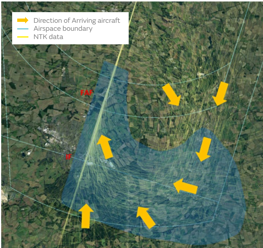
Figure 31: RWY 02 Expected Swathe for the RNAV IAPs
